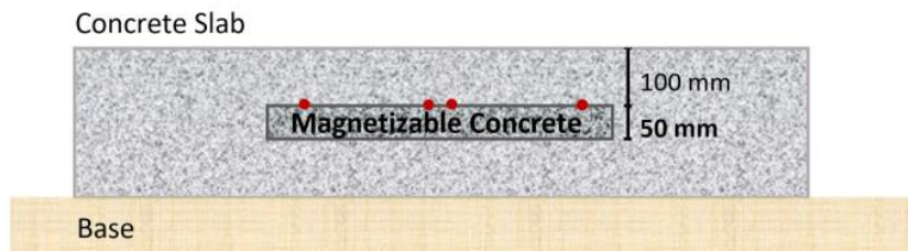
Figure 6. Cross section of Magment's inductive embedded coils
